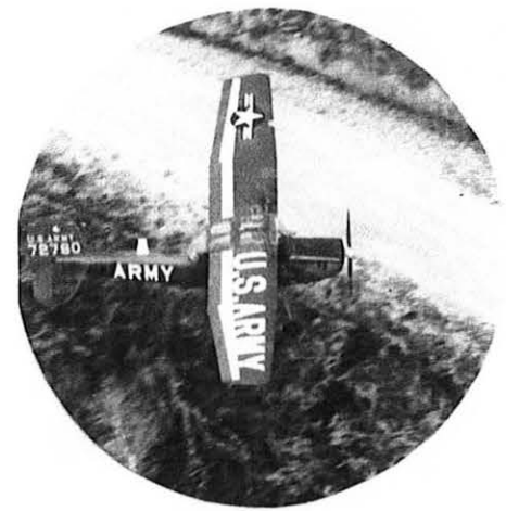
Aircraft Painting on top of wings intended for easy identification by aircraft flying above them.
