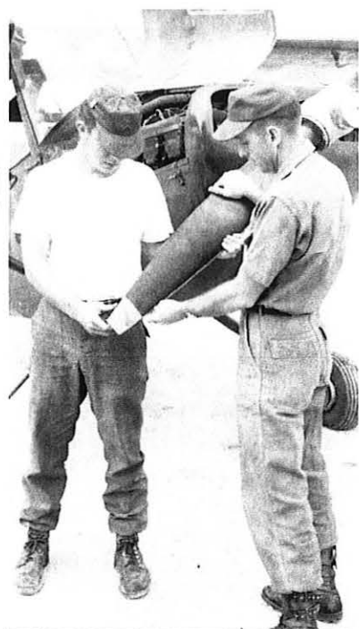
SP4 Crommett and Sgt. Goff inspect the propeller blade for chips.
