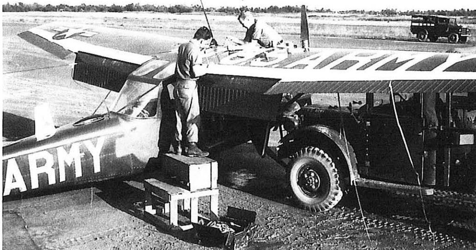
A leaky fuel tank replaced on-the-spot.
