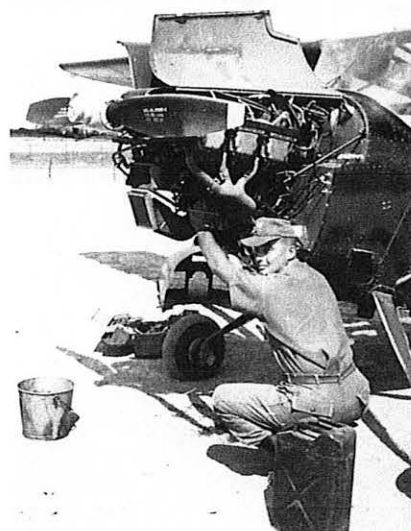
Sp4 Burns in the process of performing an intermediate inspection on one of the Section's aircraft.
