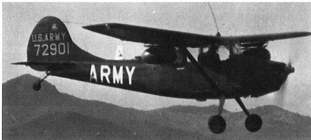
The Company's primary Aerial Photography Aircraft equipped with dual KS-54A Camera system was responsible for many valuable airphotos used to detect Viet Cong positions.
